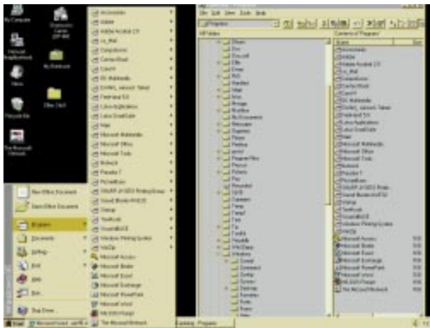
Here you can see that the files and folders showing in the Start Menu folder in the Windows directory are mirrored in the menu itself. So, you can edit the menu directly from Explorer
